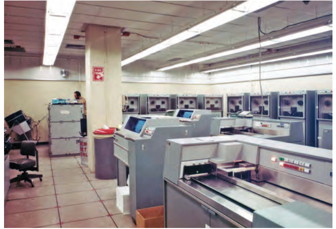
Historic view of the Tape Handler room. Line printers are in the foreground. Hard disk drives to the rear left, and tape drives to the right. Provided by Clint Esciklsen
